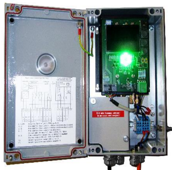
Figure 3: Configuration of EKX-4 in gas hazardous areas with opened enclosure and power switched on
